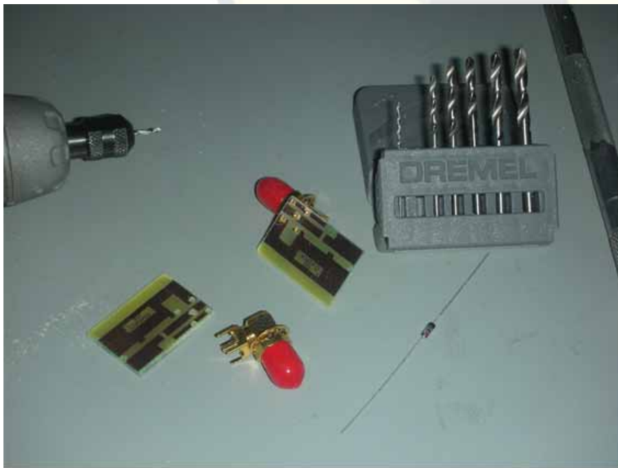
Installing SMA connectors. Use small drill bits and something like an X-acto knife to mark the PCB with the drill pattern. I made these holes by holding a dremel in hand although a press would be better. The connectors are typical edge mount types.
