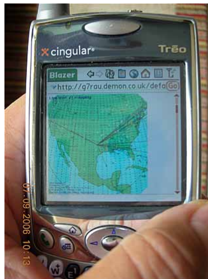
Fig 1. Live MUF V7 web version displayed on a cell phone with internet connection.
