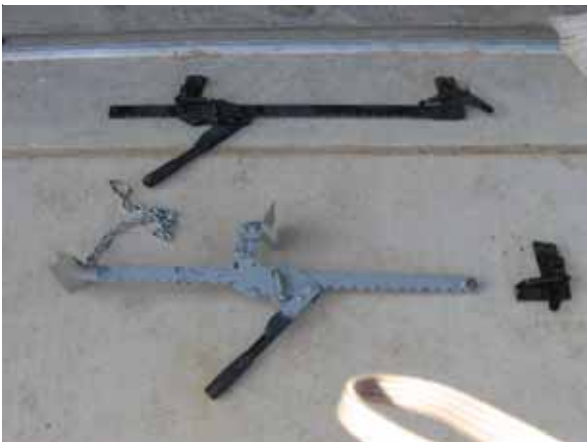
$25 fence stretcher (above) + 2 pieces of angle iron + scrap chain=tower jack (below).
