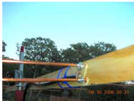
Coax is soldered directly to driven element.
