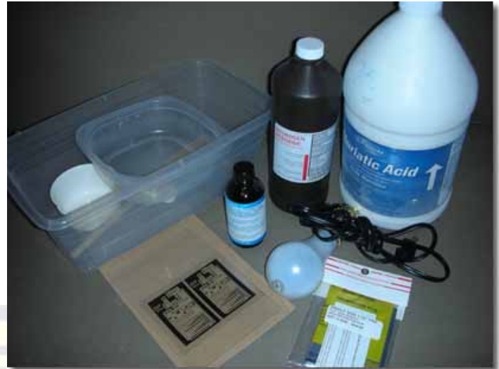
Materials required. Transparency Film on the left, Presensitized board on right.
