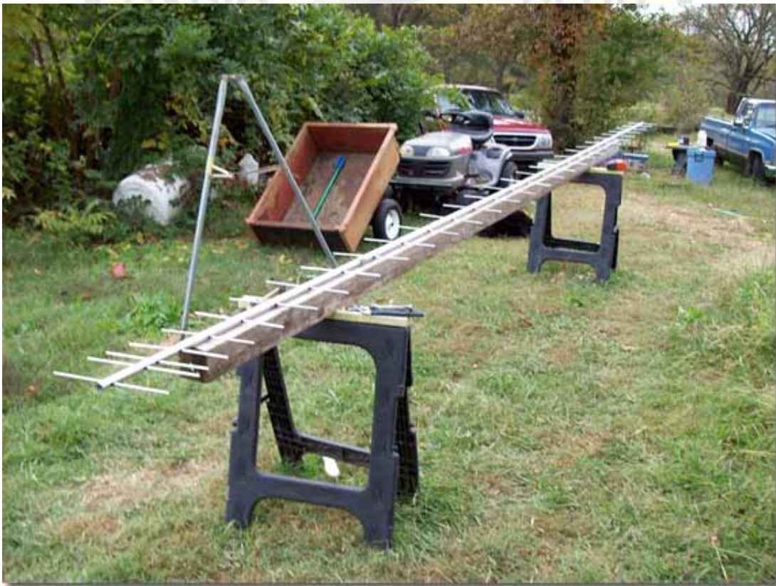
New 30 element 22 ft. long yagi constructed by Jimmie KD5ZVE, SWOT Net Manager and NCS of the Eastern Oklahoma SWOT Net which meets 8pm local on Tuesdays. The yagi has a gain of 19.55 dBi and F/B of 26 dB. Design comes from ARRL Handbook.
